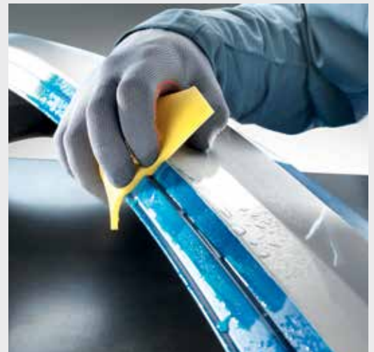
Manual sanding of contours and edges e.g. wet matting of painted car body parts
